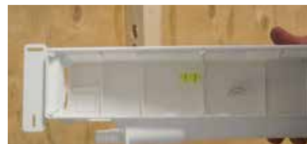
3. Place bubble level in its housing
